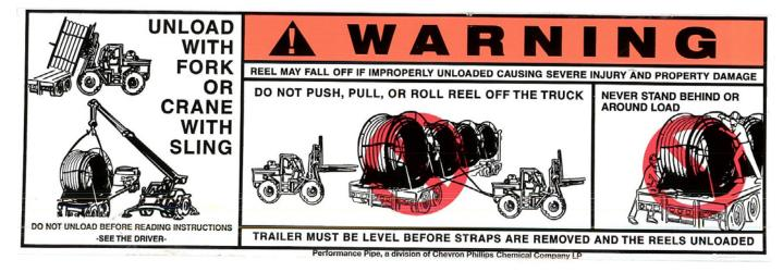
FOR METAL REELS. ATTACH THE LABEL TO THE SIDE OF EACH PIPE COIL INSIDE THE REEL.
