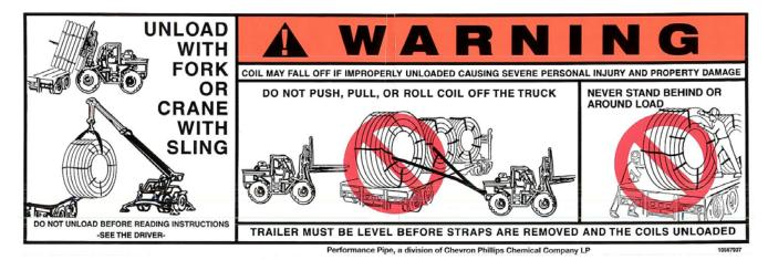
FOR VERTICAL COILS, TWO LABELS ARE TO BE ATTACHED TO ONE COIL ON BOTH SIDES OF THE TRUCK.
