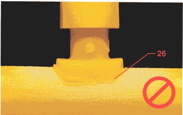
26. Gap due to incomplete melt resulting from misalignment
