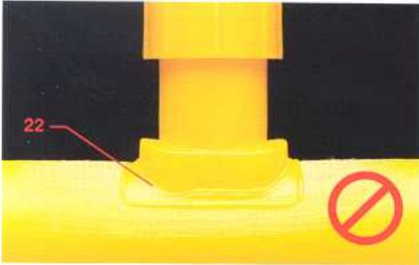
22. Melt bead too small and insufficient fusion pressure
