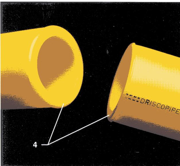
4. Proper melt ends after heat soak
