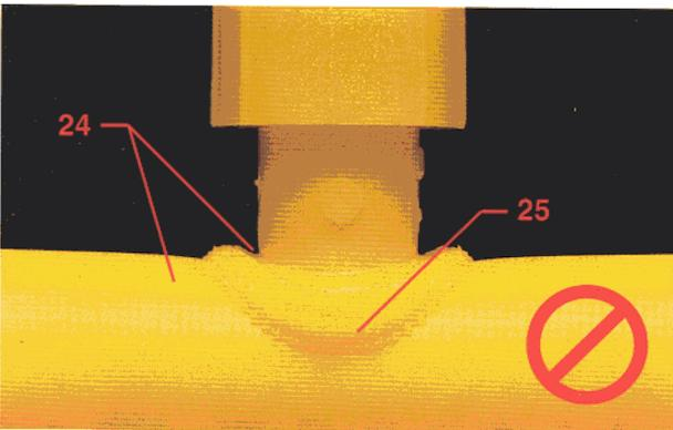
24. Melt bead is above base of fitting; Main not prepared
