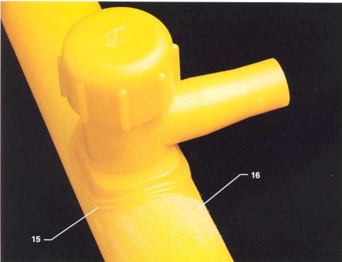
15. Proper melt, pressure and alignment.
