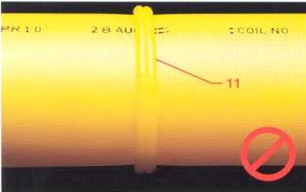
11. Excessive melt and/or excessive pressure
