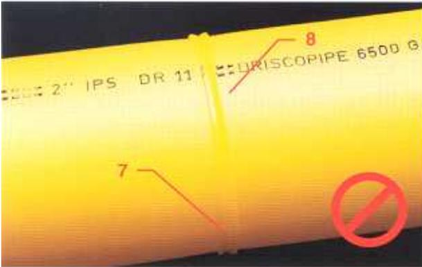
7. Insufficient fusion pressure – “V” shaped melt appearance
