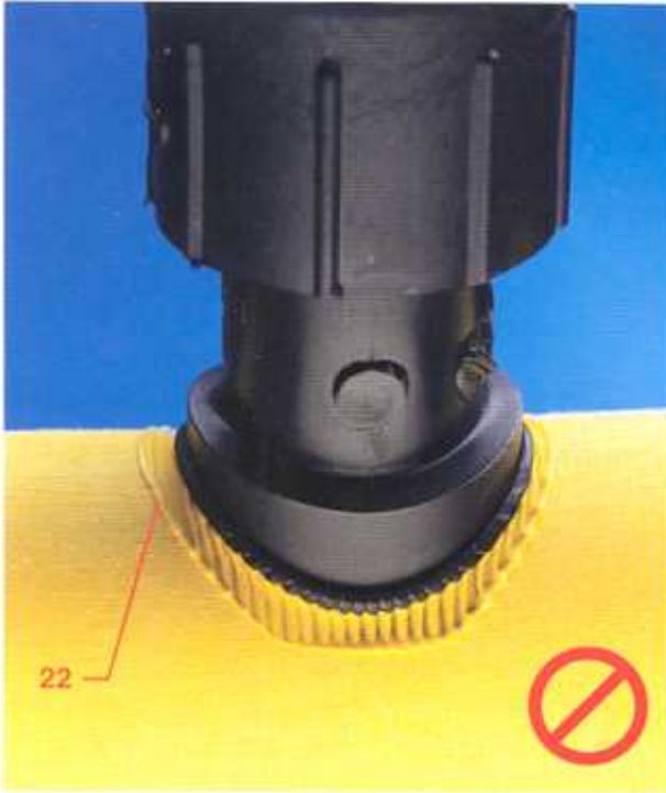
Sidewall Fusion 1 1/4 Inch Pipe: Unacceptable Appearance: Insufficient Melt
