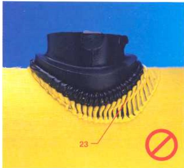
Sidewall Fusion 2 Inch or Larger Pipe: Unacceptable Appearance: Misaligned
