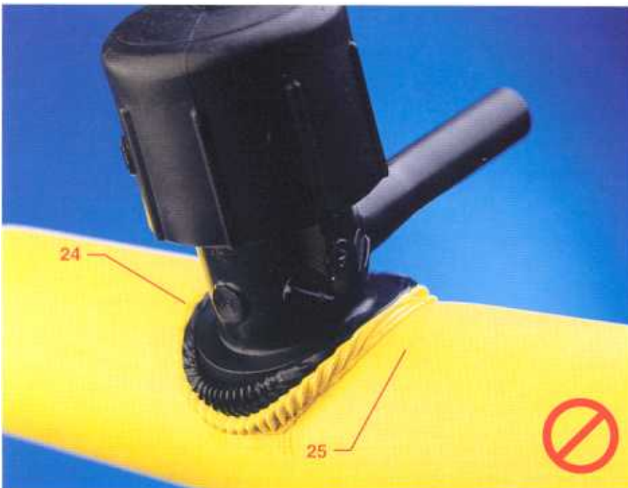
Sidewall Fusion 2 Inch or Larger Pipe: Unacceptable Appearance: Excessive Melt and Pressure
