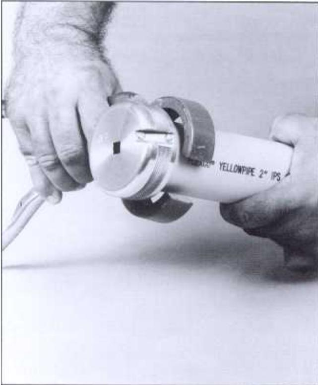
3. To measure proper socket insertion depth, place Depth Gauge snugly over the chamfered end of the pipe.
