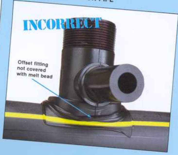
17 POOR ALIGNMENT — FITTING NOT SQUARE ON PIPE
