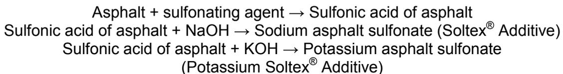
It should be pointed out that all available double bonds from hydrocarbons are eliminated by the sulfonation process used to make Soltex<sup>®</sup> Additive. An excess amount of sulfonating agent is used to guarantee the complete sulfonation and smooth processing in the plant. This process is routinely monitored by testing the solubility of Soltex<sup>®</sup> Additive and Potassium Soltex<sup>®</sup> Additive in water.
