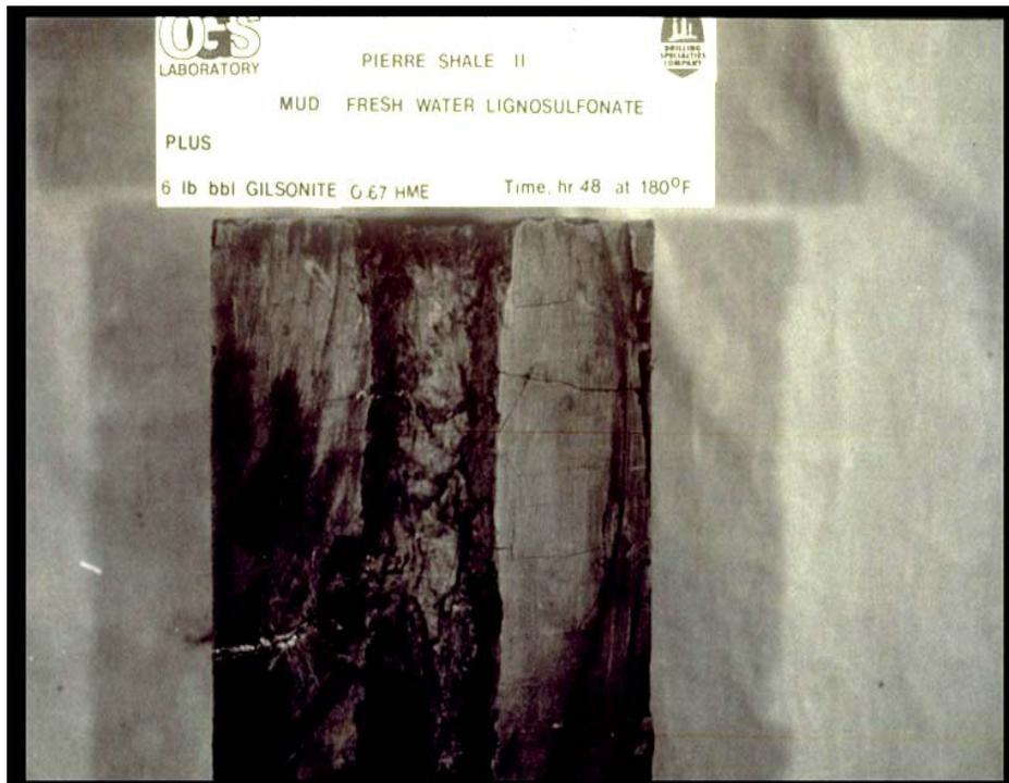
**PIERRE SHALE II DRILLED WITH A 3.2 cm MICRO BIT WASHED OUT TO 3.5cm, <10 % HOLE ENLARGEMENT TREATED WITH 6 PPB SOLTEX<sup>®</sup> ADDITIVE**
