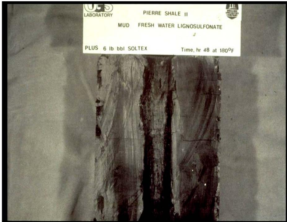
Soltex<sup>®</sup> Additive was developed for shale control. When shales fracture, the edges are more positive than the faces, thus micro-fractures in shales represent small lines of positive charge. These are bound together by the electro-negative Soltex<sup>®</sup> Additive in solution, thus inhibiting disintegration of the shale. See photo on page 8.
