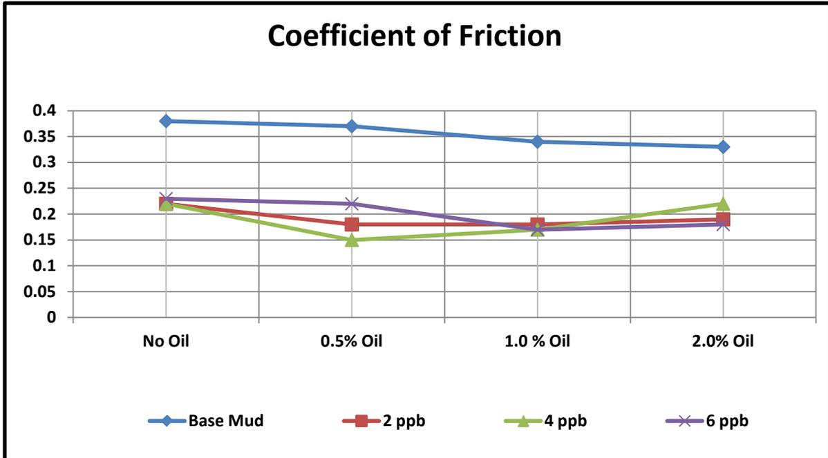
Mud samples were hot – Rolled 16 hours at 176F. The base mud = 10 ppb bentonite in fresh water, de-sanded with a U.S. standard sieve series No. 200
