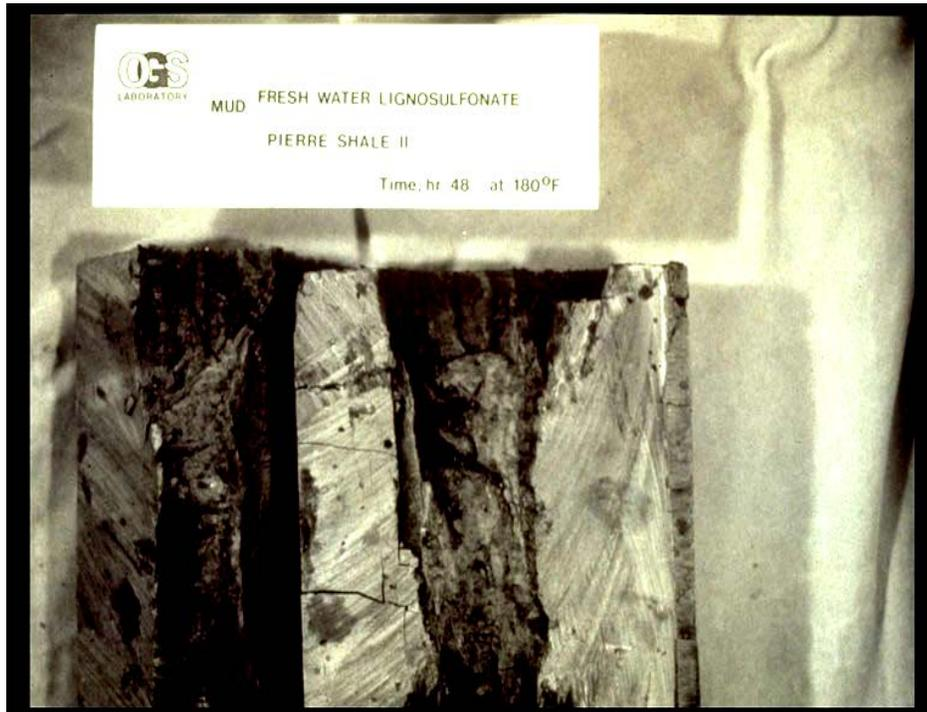
**PIERRE SHALE II DRILLED WITH 3.2 cm MICRO BIT WASHED OUT TO 4.9cm 53 % HOLE ENLARGEMENT TREATED WITH 6 PPB GILSONITE**
